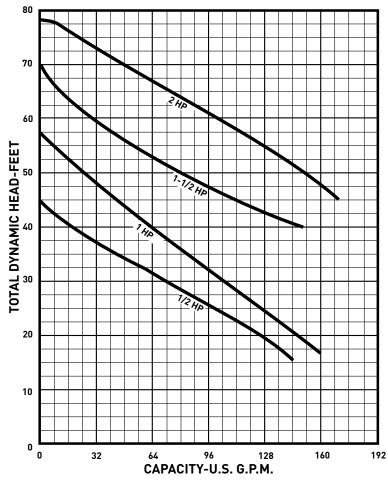
The curves reflect maximum performance characteristics without exceeding full load (Nameplate) horsepower. All pumps have a service factor of 1.2. Operation is recommended in the bounded area with operational point within the curve limit. Performance curves are based on actual tests with clear water at 70° F. and 1280 feet site elevation.
