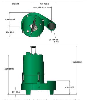
All dimensions in inches. Metric for international use. Component dimensions may vary  $\pm$  1/8 inch. Dimensional data not for construction purpose unless certified. Dimensions and weights are approximate. On/Off level adjustable.
