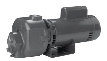
The DMC Multi-Stage Centrifugal Pump offers heads to 175 feet and capacities to 50 GPM. Designed for the professional with heavy-duty cast iron pump case and seal plates and diffuser with Noryl® impellers for years of proven service. Available in 2 HP model.
