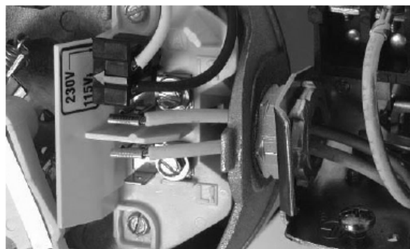
Figure 7: Voltage set to 115 V, Plug Type
