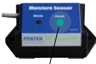
Fig. 1 Green "Ready" Indicator Illuminated
