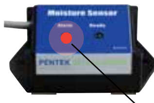
Fig. 2 Red "Alarm" Indicator is illuminated if water is touching the two detection points on the bottom of the Moisture Sensor.
