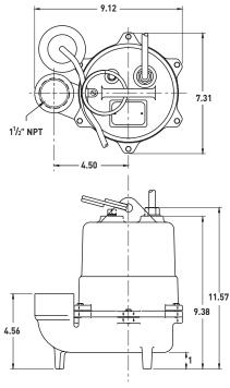
All dimensions in inches. Metric for international use. Component dimensions may vary ± 1/8 inch. Dimensional data not for construction purpose unless certified. Dimensions and weights are approximate. On/Off level adjustable.
